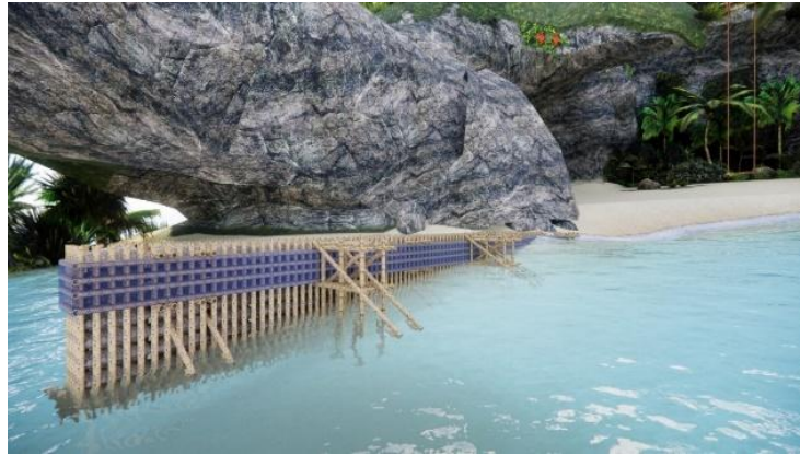
Figure 4. The three-dimensional (3D) of breakwater
